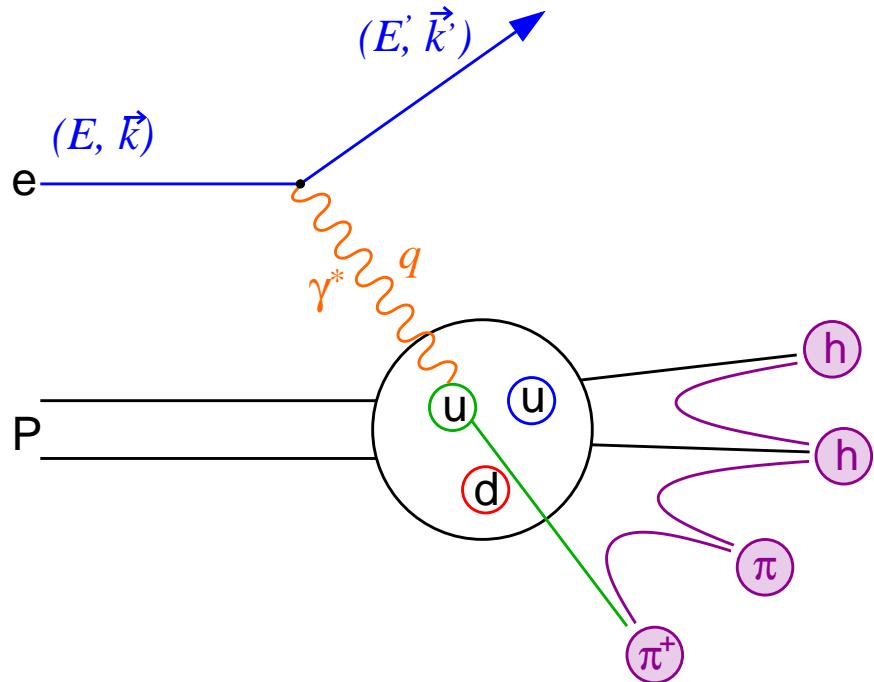
$$\begin{aligned} Q^2 &= -q^2 = -(k - k')^2 \\ \nu &\stackrel{\text{lab}}{=} E - E' \\ x &= \frac{Q^2}{2M\nu} \\ z &\stackrel{\text{lab}}{=} \frac{E_{\text{had}}}{\nu} \end{aligned}$$
